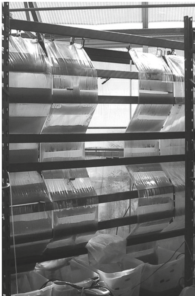
Fig. 7.5 Accordion photobioreactor developed at the University of Arizona (USA) (Courtesy of Prof. JL Cuello)
