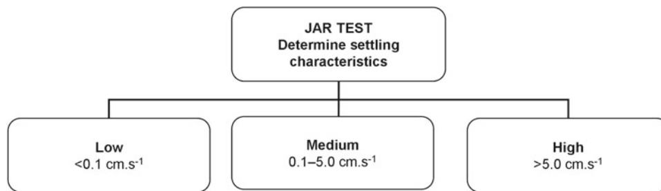
Fig. 10.20 The settling characteristics can be determined by a jar test
