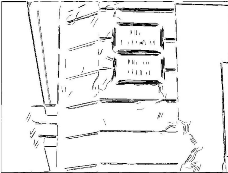
Fig. 3.4 Flat parts detection: Bretagne . 1004 detections. Flat parts as small as the ones in the letters of the name of the street are detected (about 10 pixels high). Flat parts in the boundaries of the shadows can be eliminated by dropping the probability threshold, as can be seen on Fig. 3.5. Nevertheless these detections actually correspond to small flat parts
