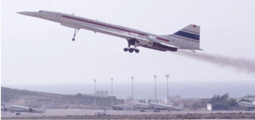
Fig. 3 At 10 h 08 Universal Time on 30 June 1973, the prototype Concorde 001, registration F-WTSS, took off from Las Palmas airport in the Canary Islands to meet up, somewhere over West Africa, with the Moon's shadow, already slipping rapidly over the Earth's surface. The afterburn (or reheat) of the four engines has been activated to get the 136 tonne airliner off the ground. © Jim Lesurf
