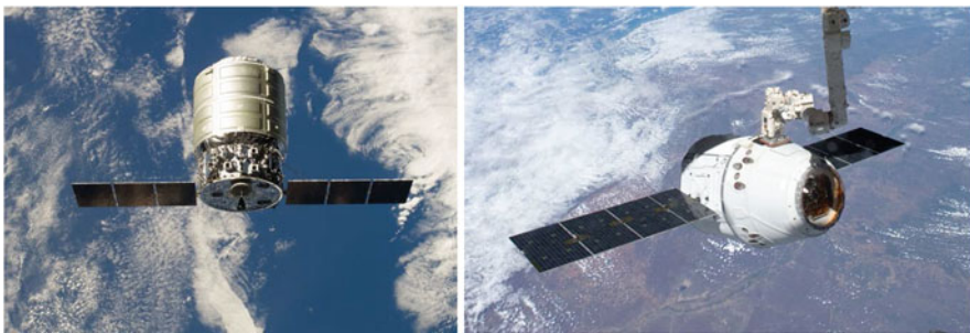
Fig. 1 The first Cygnus commercial cargo spacecraft built by Orbital Sciences Corp. is photographed by an Expedition 37 crew member on the International Space Station during rendezvous and docking operations and SpaceX Dragon cargo grappled by the Canadarm (Credit: NASA)
