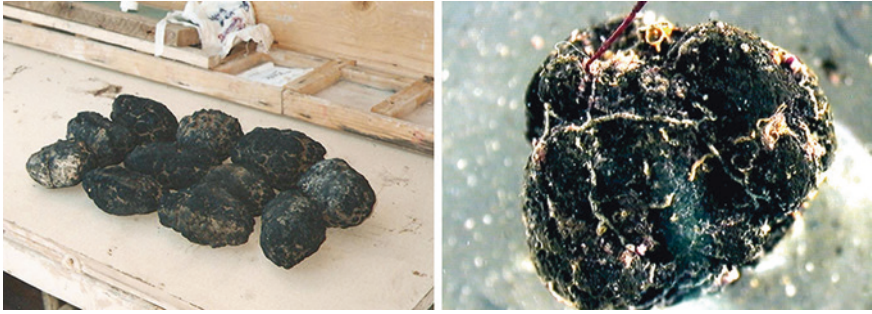
Fig. 1 Left Polymetallic nodules from the sub-equatorial NE Pacific’s Clarion-Clipperton Fracture Zone (CCFZ) on the ship’s deck, assembled for analysis (Photo T. Radziejewska); Right a close-up of a polymetallic nodule, with abundant epifauna (Photo B. Wawrzyniak-Wydrowska)
