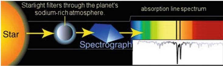
FIG. 2 Absorption spectroscopy diagram (Credit: NASA/STSCI)
