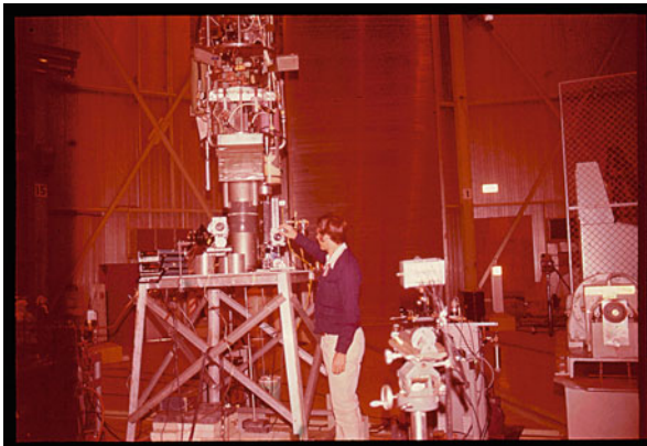
Russell De Young at the Aberdeen Fast Burst reactor where nuclear laser experiments were carried out. The reactor is shown between two test laser setups. One is the Box Laser and the other is polyethylene (neutron moderator) covered cylindrical gas tube laser.
