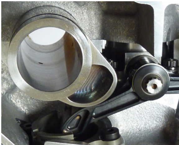
A typical finger follower cam mechanism for a high performance engine
