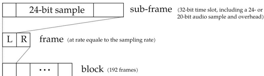
**Fig. A.1** A simplified representation of the AES3 or AES/EBU data format and time multiplexing
