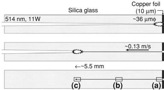
**Fig. A.3** Migration process of platinum particle (diameter:  $\sim 5 \mu\text{m}$ ) in borosilicate glass by CW-LBI [3]; (*top*) initiation, (*bottom*) propagation and termination
