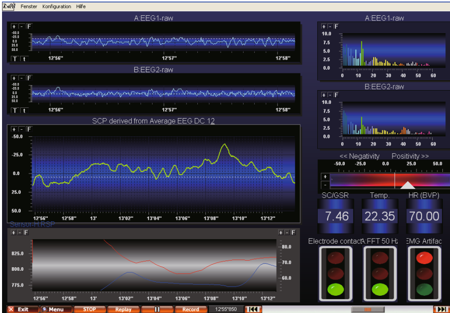
Fig. 10.7 Screenshot of the recording software Biograph. On the left: 2 channels raw EEG, SCPs, abdominal breathing extension (blue) and heart rate (red). On the right: Frequency spectrum of the 2 channels EEG, negativity-positivity slider, numbers of skin conductance level, finger temperature, heart rate, control lights for electrode, 50 Hz noise and EMG artifact. At the presented moment an EMG artifact is detected, therefore the light is red.
