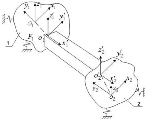
Fig. A.1 Three-dimensional finite beam element and its local coordinates systems
