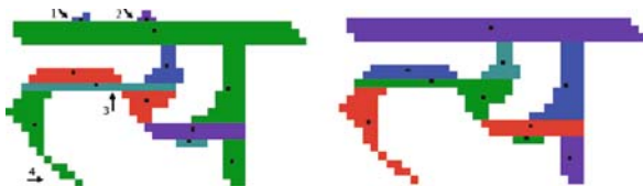
Plate 10 Illustration of BAG-based noise removal – Left: (1, 2) sample with noise, (3) thin joint, (4) thin ligature boundary; Right: result of BAG-based noise removal [10] (See also Fig. 5 on page 290)
