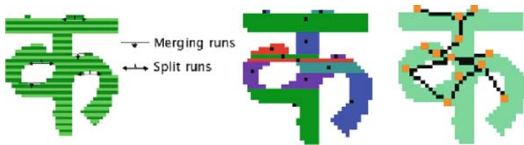
Plate 9 BAG construction using horizontal runs for a sample grapheme [10] (See also Fig. 4 on page 289)
