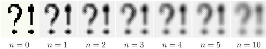
Figure A.6. Example of results with the scheme (A.67) at different times (iterations), as applied to a simple and small image (32 × 32).
