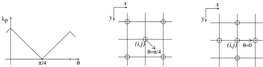
Figure A.11. Adaptive choice of the coefficients  $(\lambda_p, \lambda_d)$  as a function of  $\theta$ , the orientation of  $\nabla v$ . The two right-hand figures show which points will be used in the discretization of the divergence term in two specific situations.
