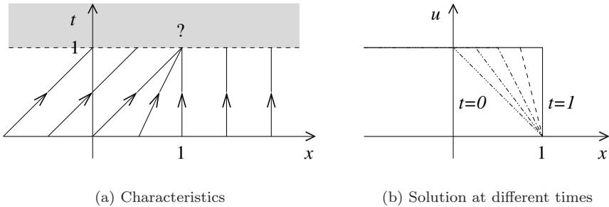
Figure A.4. Behavior of the Burgers equation (A.49). The left-hand figure represents the characteristics while the right-hand one shows some solution at different times. As we can observe, characteristics intersect at  $t = 1$ , and after this time, it is not clear how to define the solution.
