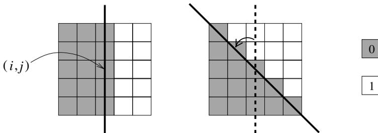
Figure A.7. Example of a binary image representing a vertical edge and the same image after a rotation of  $\pi/4$  radians. Rotationally invariant operators estimated at the point in the middle should yield the same value in both situations.
