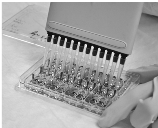
Fig. 5. Photograph of an IdMOC multi-well plate with sixteen chambers and six inner wells per chamber (IdMOC-96). The plate has the same footprint of a regular 96-well plate and is compatible with multi-channel pipets.
