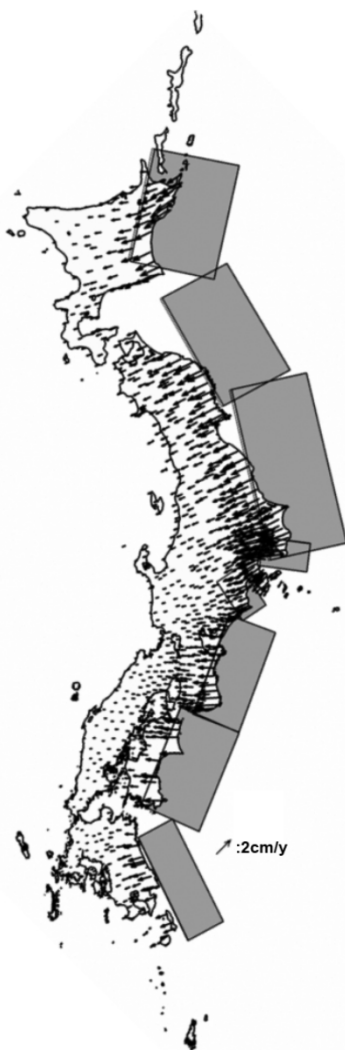
Fig. A.1. Rectangular faults assumed for calculating crustal deformation caused by the subducting oceanic plates. The arrows show accumulating horizontal displacement rates.
