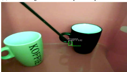
Fig. 17 (a–b) False negatives and IoUs for detected instruments for each of the other backgrounds, for a model trained on images from all backgrounds (including the original simulator box). Note that the scale
