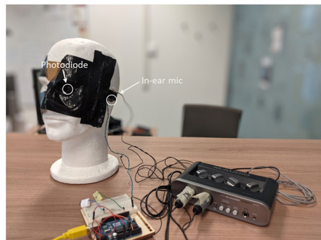
Fig. 10 Apparatus used for the characterization of the VR stimulus' audio-visual properties
