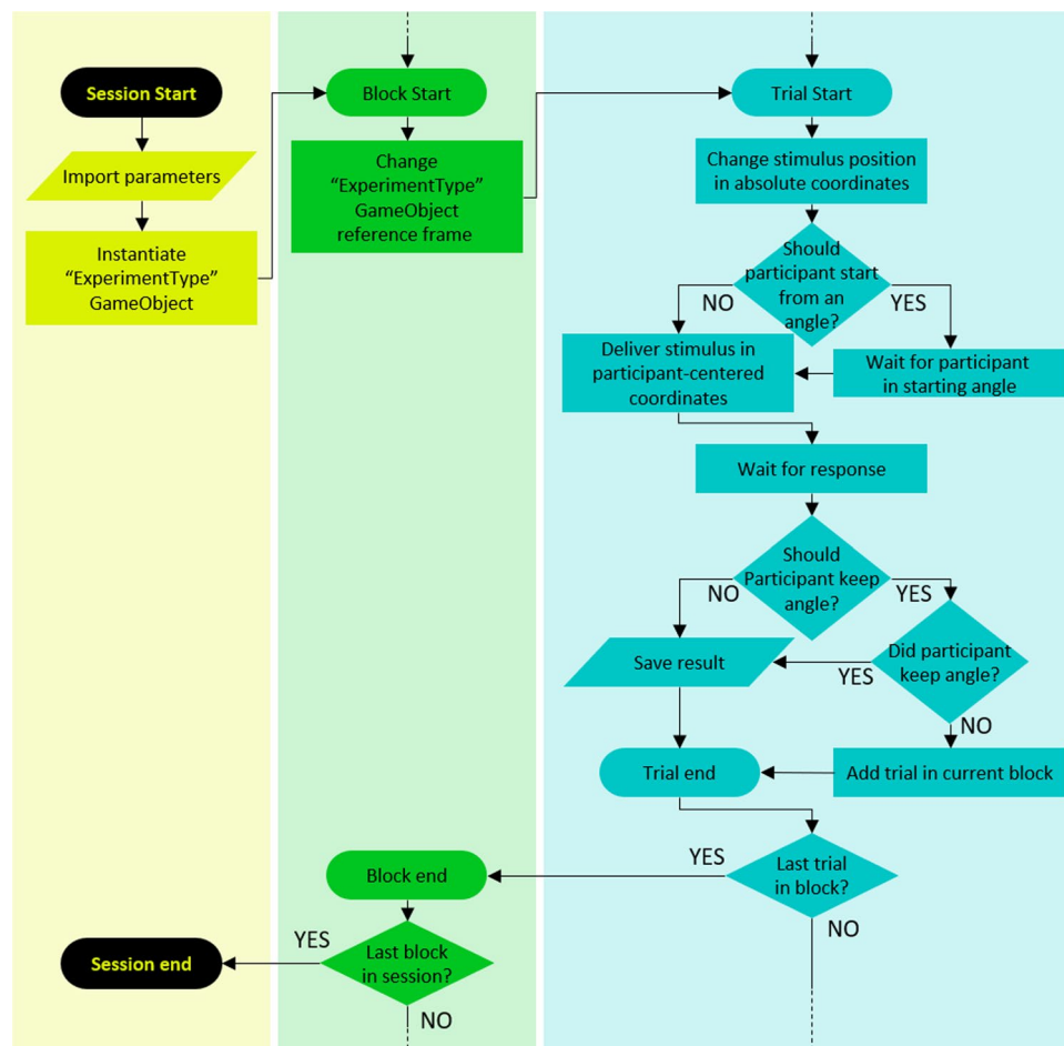
Fig. 5 Flowchart outlining the events that compose an experiment using SALLO and UXF. The UXF events trigger the SALLO-based stimuli delivery. The SALLO-based stimuli delivery does not strictly depend on UXF but can be triggered using any other Unity asset based on events
