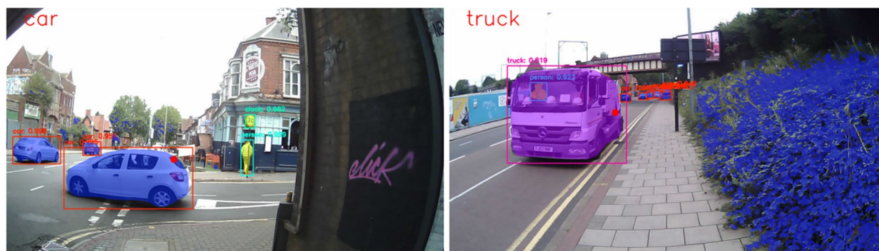
Fig. 3 Screenshots of the system’s output video complete with greenery masks (blue), labeled objects, gaze overlay, and “gazed upon” object label. An example of video footage can be found in Yeo (2020)
