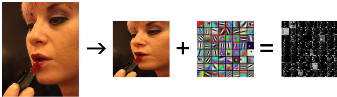
Fig. 4 A visualization of the weights of the first layer of AlexNet. The image (left), resized to 224 \times 224 pixels, combined with the 64 filters (middle), creates 64 matrices (visualized as 64 gray-level images, right). Each filter represents some low-level feature in the processed image. We took the mean of each matrix as a measure of the content of the
