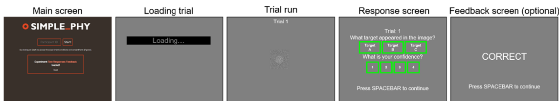
Fig. 3 Outline example of one experiment: Main screen: Where participants type their participant ID. Loading trial: A filler screen that participants see as the files necessary for each trial are loaded. Trial run: Where the trial stimuli are displayed and the participants either press a key, make a mouse click, or wait for a designated timeout when viewing
