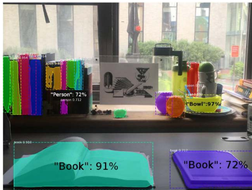
Fig. 3 Example Mask RCNN Output. Object labels and class probabilities are visible in white. The visible rectangular bounding boxes surrounding object masks are a by-product of the Mask RCNN
