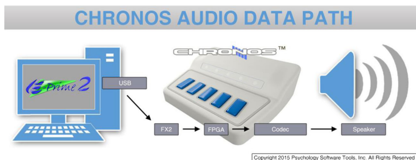
Fig. 2 The Chronos audio data path. E-Prime generates the audio data as binary data, which are then transmitted as serialized data via USB. Then, inside Chronos, the FX2 microcontroller reverses the serialized data back to binary. The field programmable gate array (FPGA) reads bulk data in from the FX2 and stores them in a buffer, which is always kept full if data
