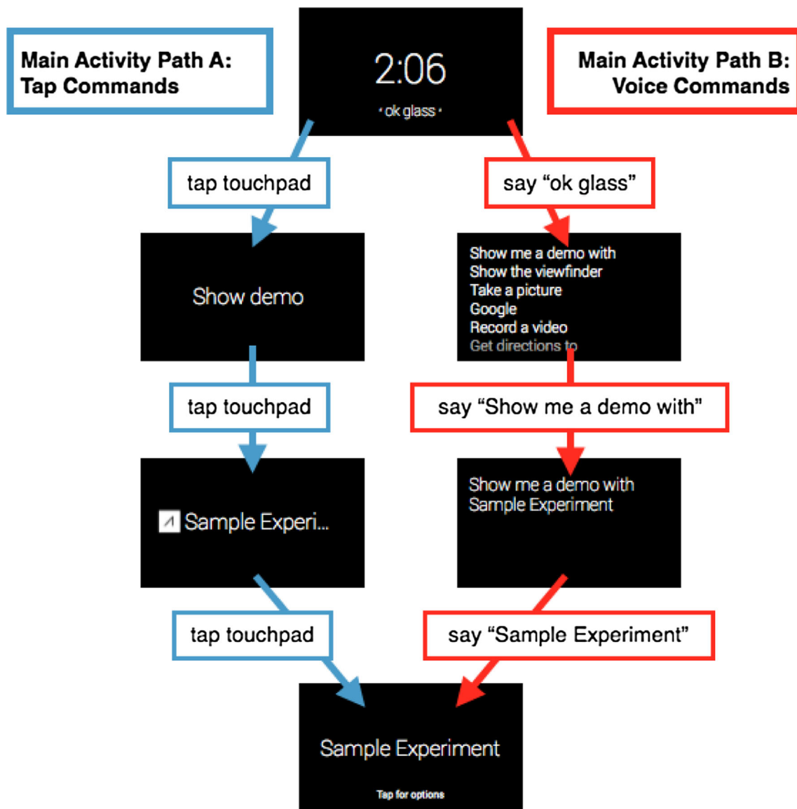
Fig. A1 PsyGlass Glassware flow for navigating to the data collection study (“Main Activity”). The Main Activity can be accessed in two ways: navigating with the touchpad (Path A) or through voice commands (Path B)
