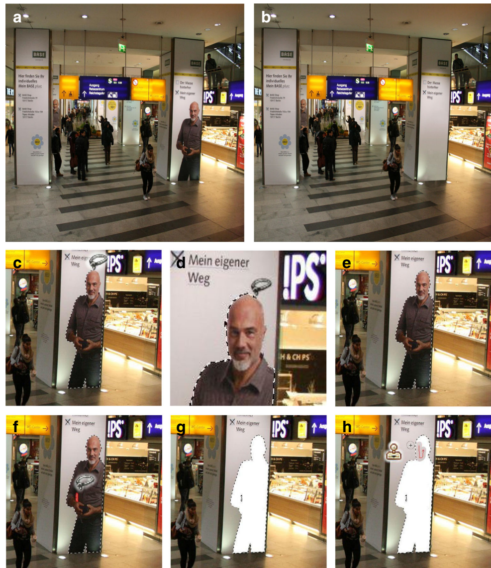
Fig. 2 Creating a deletion change, showing the original (a) and modified (b) scenes. In this example, the man on the ad is deleted from the original image. The object is selected with the Free Select tool (c) and magnified in order to increase selection precision (d). After finishing the coarse object selection (e), the selection is refined and certain areas are excluded from the selection range (red area in panel f). Next, the object is deleted (g), and the resulting empty space is filled in using the Clone tool (h)
