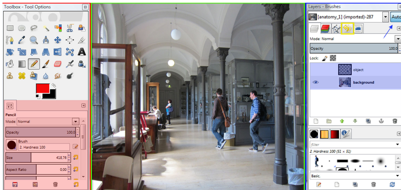
Fig. 1 Default layout of GIMP. Important windows are marked by colored squares: the Tool window with tool shortcuts (red) and specific tool information (red-shaded); the Main window (green); and the Layers
