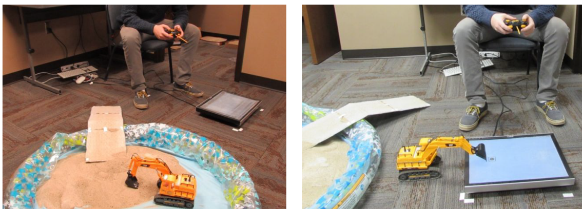
Fig. 5 Experimental setup for experiment 3. The left panel shows the excavator during the raking phase of the experiment. The participant drove the excavator in and out of the pool, so they maintained control over the excavator for the duration of the experiment. The right panel
