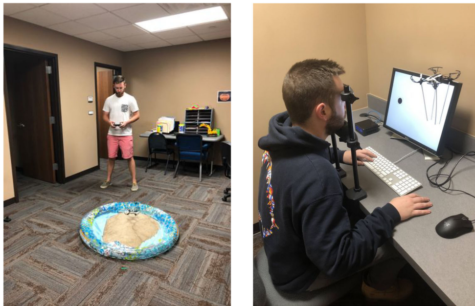
Fig. 3 Experimental setup for Experiment 2. The left panel shows a participant raking sand with the drone, by hovering the drone over the pool until the prongs extending down from the drone make contact with the sand. The right panel shows the configuration for the target-detection
