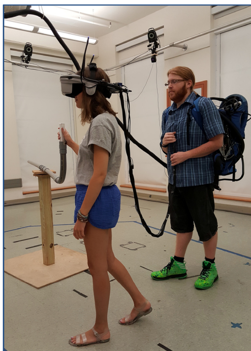
Fig. 2 Apparatus used in all experiments. Participants wore a virtual reality head-mounted display (HMD) that afforded dichoptic stimulation, and, on some trials they walked at a natural pace around a large, circular path, walking either forward or backward for the duration of a given trial, and pressing keys on a response box to indicate rivalry dominance. The control pack interfacing the display and response box to the computer was worn by an experimenter who trailed the participant while walking. No participant complained about the task or expressed discomfort walking forward or backward in this manner
