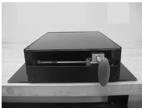
Fig. 1 Manipulandum used to execute actions with objects in the learning phase and to execute actions with a cylinder during the experimental phase. A hollow rod (placed to the right) allowed the experimenter to mount the different objects or the cylinder
