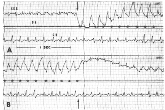
Fig. 2. A polygraph record showing the presence or absence of artifacts in the electrocardiogram (EKG) when drinking is monitored with a drinkometer (DR) or a crystal (CR), respectively. The drinkometer was turned on at the downward arrow and off at the arrow pointing up.
