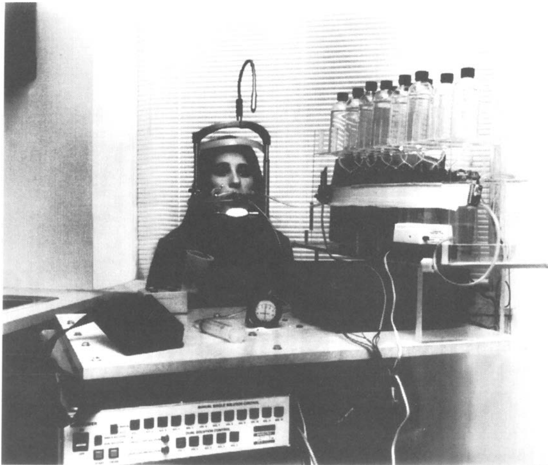
Figure 1. The University of Pennsylvania Regional Automated Taste Testing System (RATTs), with the subject seated comfortably and the glass stimulation device, a suction gauge, and the microprocessor in place. The table can be moved up or down electrically to accommodate the subject's height. The flexible extension from the top of the headrest contains a light that cues stimulus delivery.
