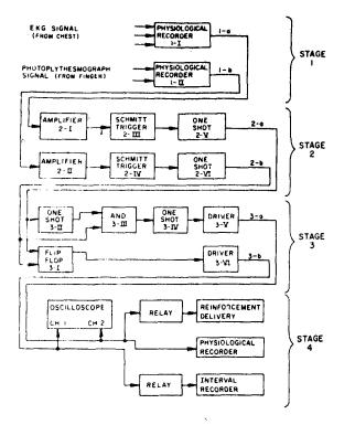
Fig. 1. Overall block diagram of the measurement apparatus.
