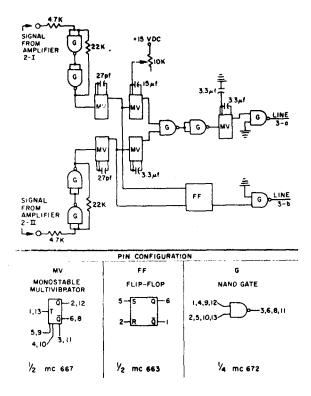
Fig. 3. Circuit diagram of Stages 2 and 3 (with the exception of information contained in Fig. 2). All integrated circuits are Motorola Type MHTL. Resistors are  $\frac{1}{2}$  W, 10%. Capacitors in microfarad range are solid tantalum, 20%, and capacitors in picofarad range are mica, 10%.
