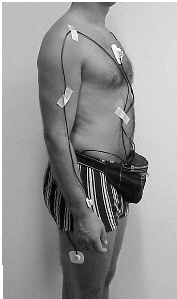
Figure 1. An extended configuration of the Activity Monitor, with accelerometers at the thighs, trunk, and lower arms.
