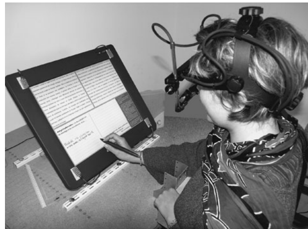
Figure 3. EyeLink2 eye tracker with Wacom 18sx screen tablet. The head is free, and the tablet is set at an angle of 50°.
