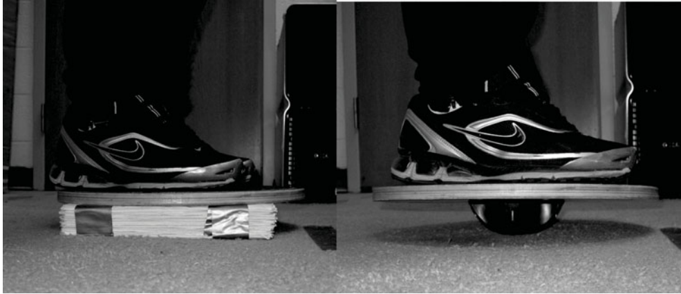
Figure 2. Participants judged the width of the beam while both balanced (left) and unbalanced (right). In the unbalanced condition, the balance board rotated about its center point. The participant was instructed to keep the board horizontal.
