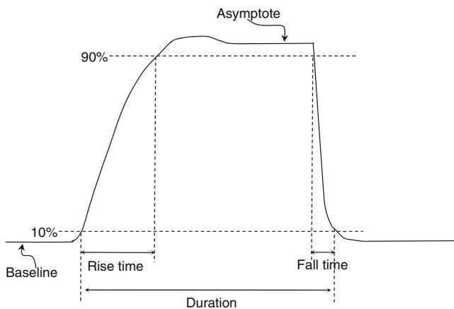
**Fig. 6** Schematic representation of the method of calculating the rise time, fall time, and duration of the displays on the LCD screen
