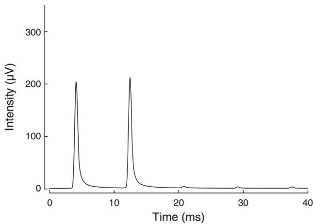
**Fig. 4** Luminance changes produced by a white bar displayed for two refresh cycles on a CRT screen running at 120 Hz. Represented on the ordinate is the strength of the illumination signal (in microvolts) recorded by the photodiode
