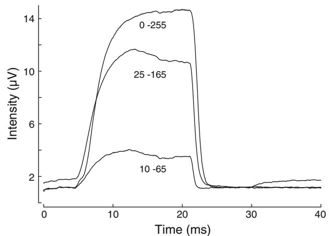
**Fig. 5** Luminance changes produced by a light bar displayed for two refresh cycles on an LCD screen running at 120 Hz. Three luminance transitions were tested: one black-to-white transition (RGB 0, 0, 0 to 255, 255, 255, labeled as 0–255), and two gray-to-gray transitions (RGB 25, 25, 25 to 165, 165, 165, labeled as 25–165, and RGB 10, 10, 10 to 65, 65, 65, labeled as 10–65). Represented on the ordinate is the strength of the illumination signal (in microvolts) recorded by the photo diode
