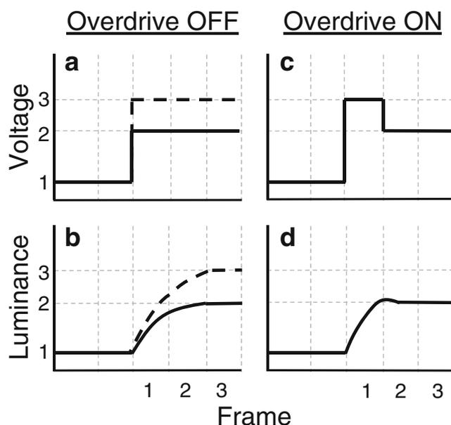
**Fig. 1** Schematic representation of the implementation of overdrive technology in LCD monitors. See the text for an explanation
