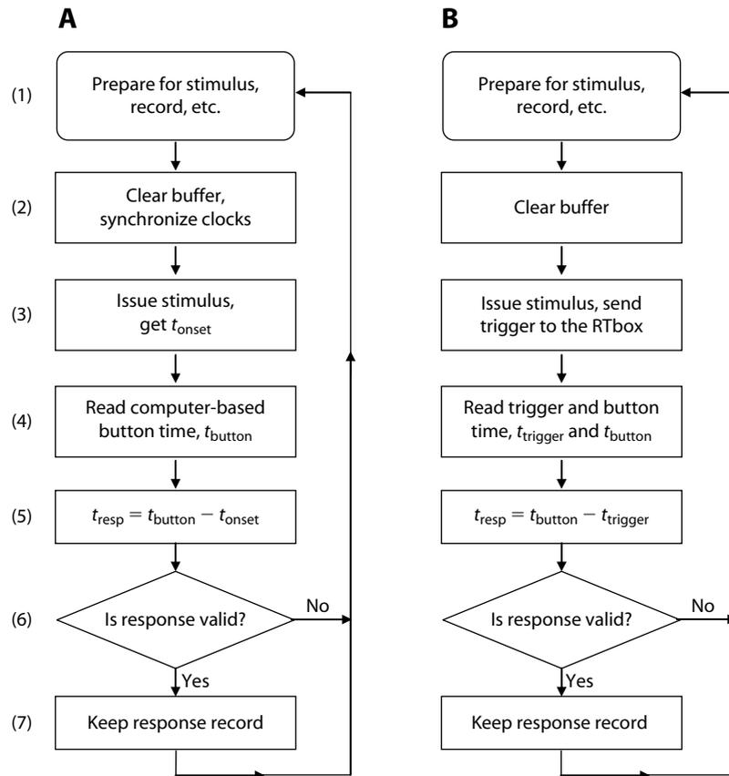
**Figure 4. Flowchart of a typical response time (RT) experiment using the RTbox. (A) Steps to measure RT without an external trigger. The button time ( $t_{button}$ ) at Step 4 is computed from the RTbox time and the clock difference measured in Step 2. (B) Steps to measure RTs using external triggers.**
