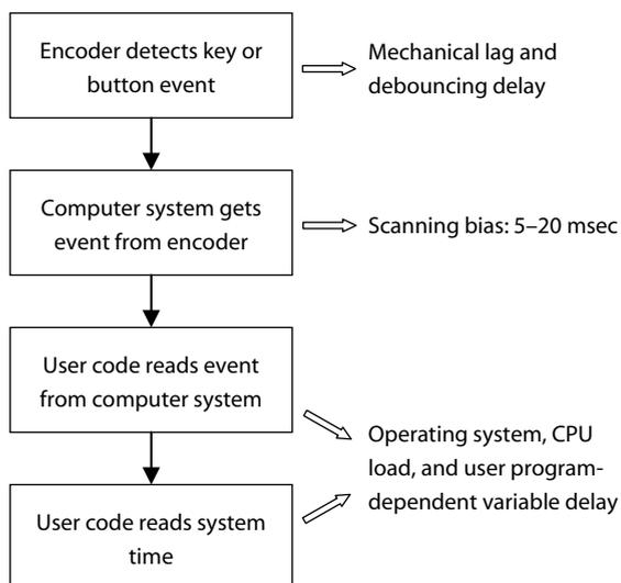
**Figure 1.** A diagram showing the steps involved in measuring response times with a regular computer keyboard/mouse. Each step may introduce some timing error, as summarized on the right side of the figure.
