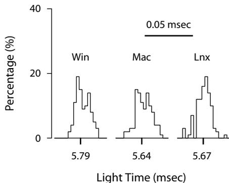
**Figure 7.** “Response time” measured without external trigger. The histogram shows the percentage of light signal time measured from the light port, relative to stimulus onset returned by the Screen(‘Flip’) function of PsychToolbox 3. One hundred trials were collected on each computer system. The tick at each horizontal axis indicates the median of the samples.
