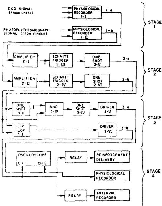
Fig. 1. Overall block diagram of the measurement apparatus.
