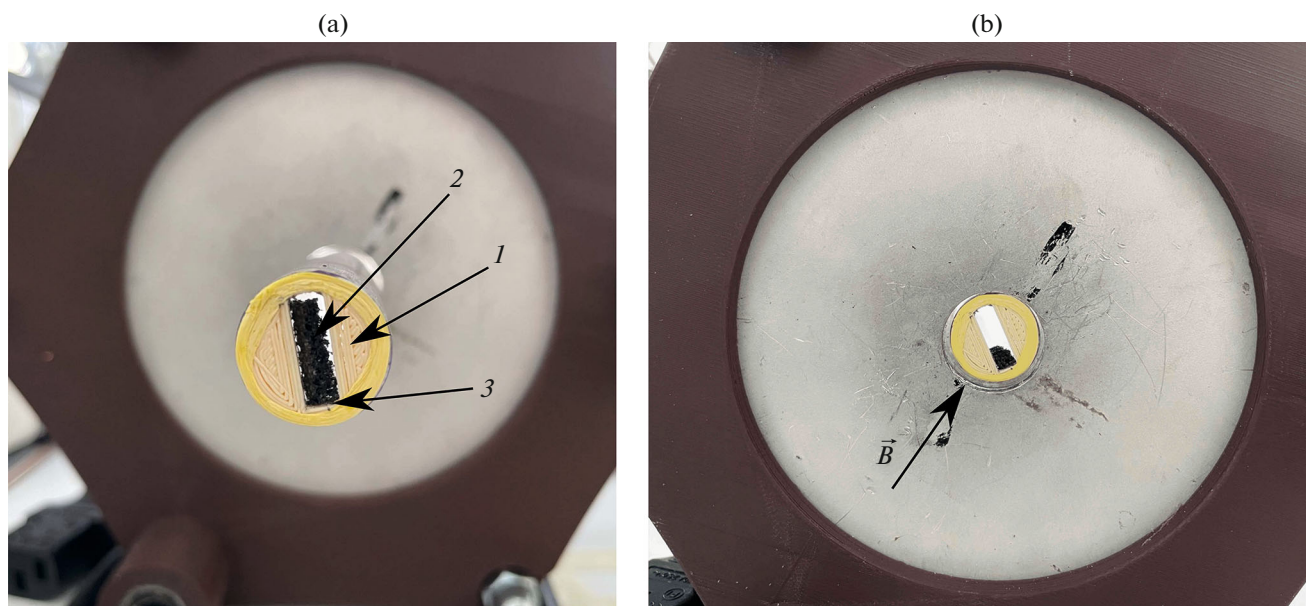
Fig. 4. Prototype demonstrating the operating principle of the magnetic field-driven valve: plastic valve base (1), porous BaFO/PDMS (2), porous BaFO/PDMS end (3) fixed to the base in (a) the closed state and (b) the open state when a nonuniform magnetic field is applied to the valve (the direction of the field is indicated by the arrow).
