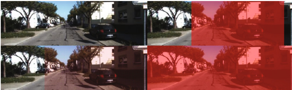
Fig. 4. The receptive field (RF) of ERFPoseNet. Top, left to right: original image from KITTI dataset, RF for baseline PoseNet. Bottom, left to right: RF for ERFPoseNet (Dilated), RF for ERFPoseNet (Dfc) and ERFPoseNet (Dfcv2). We use backprop to compute the RF and exploit the fact that the values of the weights of the network are not relevant for computing RF. We change the weight for every layer to be 0.05 and the bias to be 0. To create a situation in which the gradient at the output of the model depends only on the location of the pixels a white image is passed into the network. For visualization, we only compute RF for the one pixel in the first channel of the penultimate conv layer—set the corresponding gradient value to 1 and all the others to 0. When we backpropagate this gradient to the input layer and light up the RF as a red mask.
