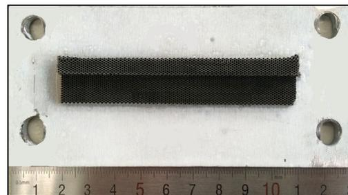
Fig. 5 Honeycomb sample used in rubbing test
