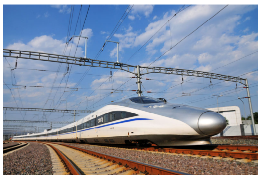
Fig. 4 CRH380A of Chinese Railways; based on Series 500 (front shape), E2 (traction system), and ICE-3 (front cabin design) totally improved by Chinese Railway designers
