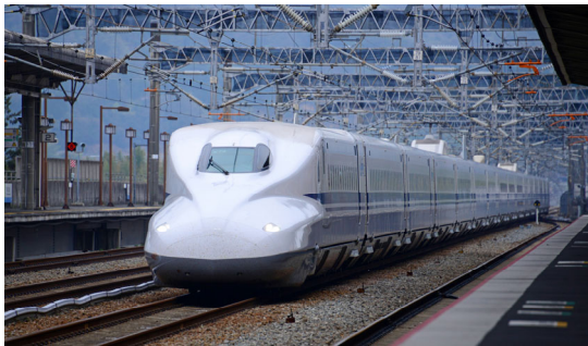
Fig. 2 Series N700 (14M2T) of Central Japan Railways; this can run at 270 km/h at 2500 m radius sharp curve by body inclination control
