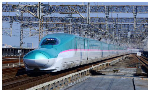
Fig. 5 Series E5 of East Japan Railways; Japan's highest speed operation at 320 km/h on 4000 m radius curve assisted by body inclination control realized together with E6, seen at the rear of the photo
