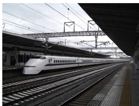
Fig. 1 Series 300 of Central Japan Railways; the world first high-speed trainset adopting regenerative braking
