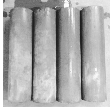
Fig. 14 Model concrete piles
