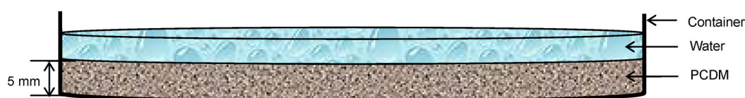
Fig. 1 Diagrammatic sketch of alkalis leachability test
