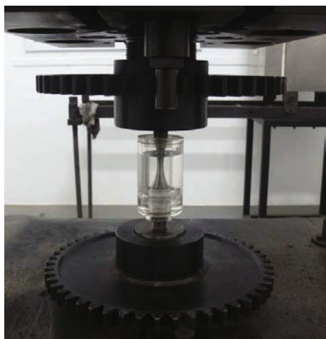
Fig. 3 Loading equipment for corrosion fatigue
