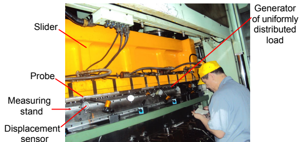
Fig. 9 Measurement of prototype's linear deflection
