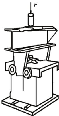
Fig. 3 Test set-up of WS specimen (DL/T 5332-2005, 2006)
