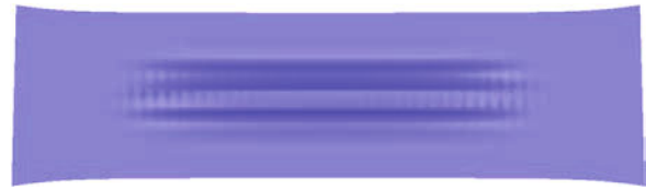
Fig. 15 Overall perspective view of the final wrinkle profile for the stretched membrane
