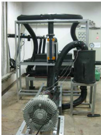
Fig. 4 Prototype of ice slurry making system
