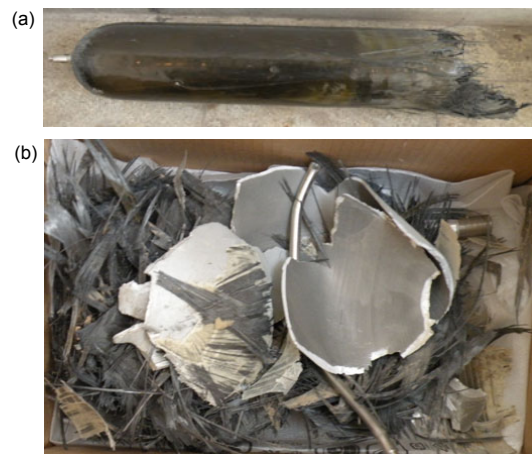
Fig. 9 Sample vessel (a) and vessel fragments (b) after bursting
