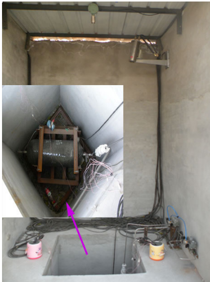
Fig. 7 Fatigue test of composite hydrogen storage vessel
