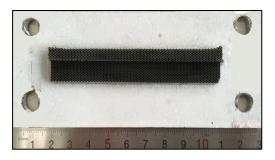
Fig. 5 Honeycomb sample used in rubbing test
